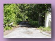
**Driveways and Access Roads -** Driveways should be built and maintained in accordance with state and local codes to allow fire and emergency vehicles to reach your home. Consider maintaining access roads with a minimum of 10 feet of clearance on either side, allowing for two-way traffic. Ensure that all gates open inward and are wide enough to accommodate emergency equipment. Trim trees and shrubs overhanging the road to allow emergency vehicles to pass.
