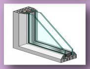
**Windows -** Heat from a wildfire can cause windows to break even before the home is on fire. This allows burning embers to enter and start fires inside. Single-paned and large windows are particularly vulnerable. Install dual-paned windows with one pane of tempered glass to reduce the chance of breakage in a fire. Consider limiting the size and number of windows that face large areas of vegetation.
